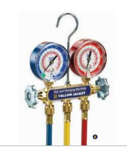
Larger, easier to read 3-1/8" color-coded gauges in rugged steel cases with polycarbonate crystals. These gauges feature 1% accuracy (Class 1) for an exact reading in critical charge systems.
